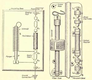
Fig. 158.—The diagram of "circuitbreaker-type" lightning protector.
